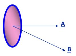
In the easiest case, with a constant magnetic field <u>B</u>, and a flat surface of area A, the magnetic flux is
