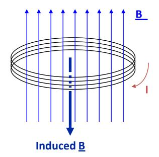
The induced EMF is  $\mathcal{E} = - d\Phi_B / dt$ Here  $\Phi_B = N(BA) = NB (\pi r^2)$ Therefore  $\mathcal{E} = - N (\pi r^2) dB/dt$ Since B(t) = 0.6t, dB/dt = 0.6 T/s
