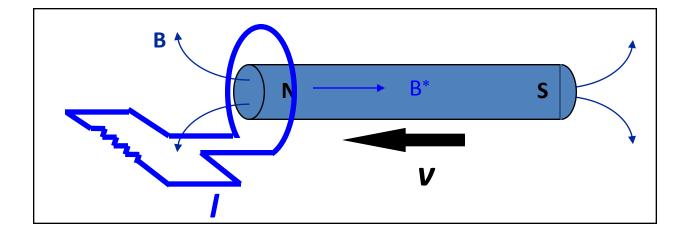
If we move the magnet towards the loop the flux of B will increase. Lenz's Law  $\Rightarrow$  the current induced in the loop will generate a field B\* opposed to B.
